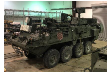
Figure 1. First ITATS Atop Army Mobile Expeditionary High Energy Laser (MEHEL) Platform
